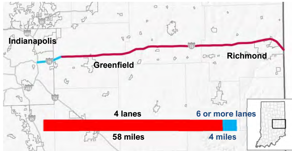
Figure 11: I-70 East Traffic Lanes
